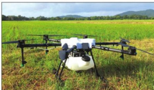
Unlike a regular drone, the agricultural drone has a diameter of 1.5m and can carry the weight of 10 litres of pesticide or 10kg of weedicide
